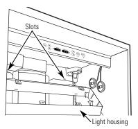
**8.** Holding up the light housing, place each lamp assembly in its holder. Feed the attached wires through the slots and tuck the wires outside the side of the light housing.
